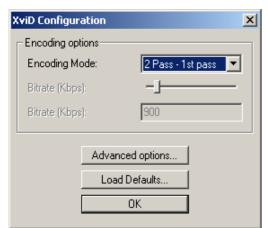
Assuming you're going to do a Two Pass encode to achieve the best results for your desired target size, select "2 Pass – 1st pass" for the first pass. Then click "Advanced options" button, which brings the "XviD Configuration" window below.
