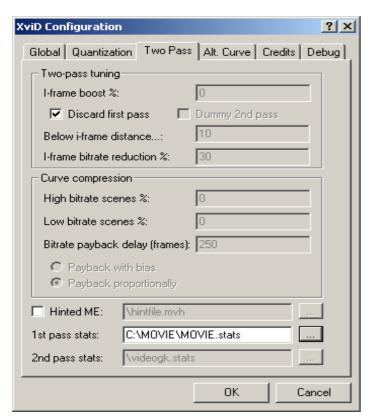
Options in "Quantization" tab are inactive for the first pass. Go to "Two Pass" tab and specify the name and location of your 1st pass stats file. Leave the rest as is and do NOT check Hinted ME.
