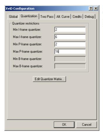
In the "Quantization" tab, cap the I-frame and P-frame quantizers as shown
